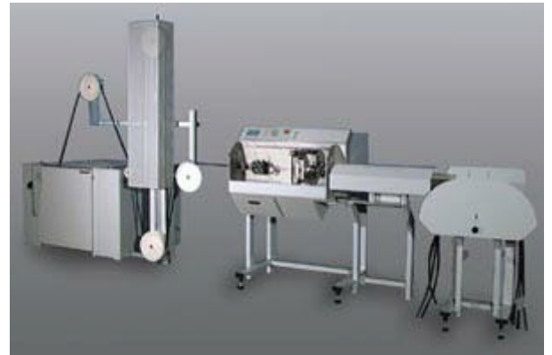
kappa 240 on production table, with komax 280 wire deposit system and de-reeler RA 800/300
